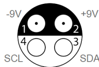
Probe’s power supply pin assignment “cable view”
